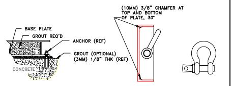
TYPICAL ANCHOR BOLT DETAIL FOR (25MM) 1.00 DIA, MOUNTING HOLE LIFT EYE 4 PLCS. NOT TO SCALE
